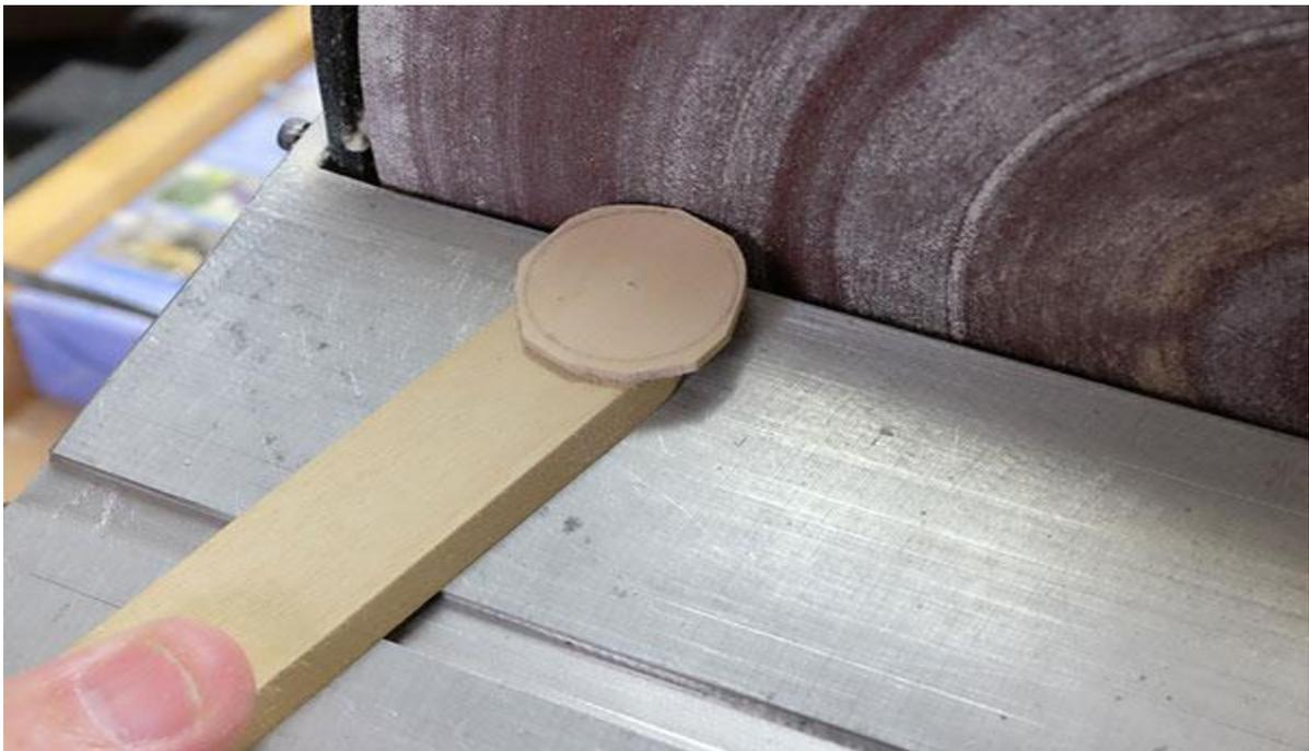
All you have to do is rotate the disk around the rod and you'll get a nice round disk. It is hard to tell, but I have the table angled down to put a bevel on the edge. You can see that bevel in the pic of the conical jig above.
