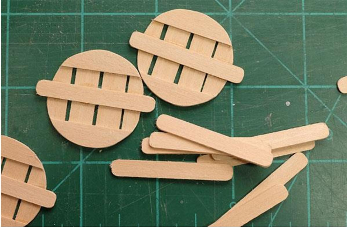
Now, you'll have to thin these down with the thickness sander. I made a simple push stick to help get them through. You'll want these pretty thin. Sand from both sides and take a couple passes per side so you can sneak up on the final thickness. Don't take all the material off from just one side.
