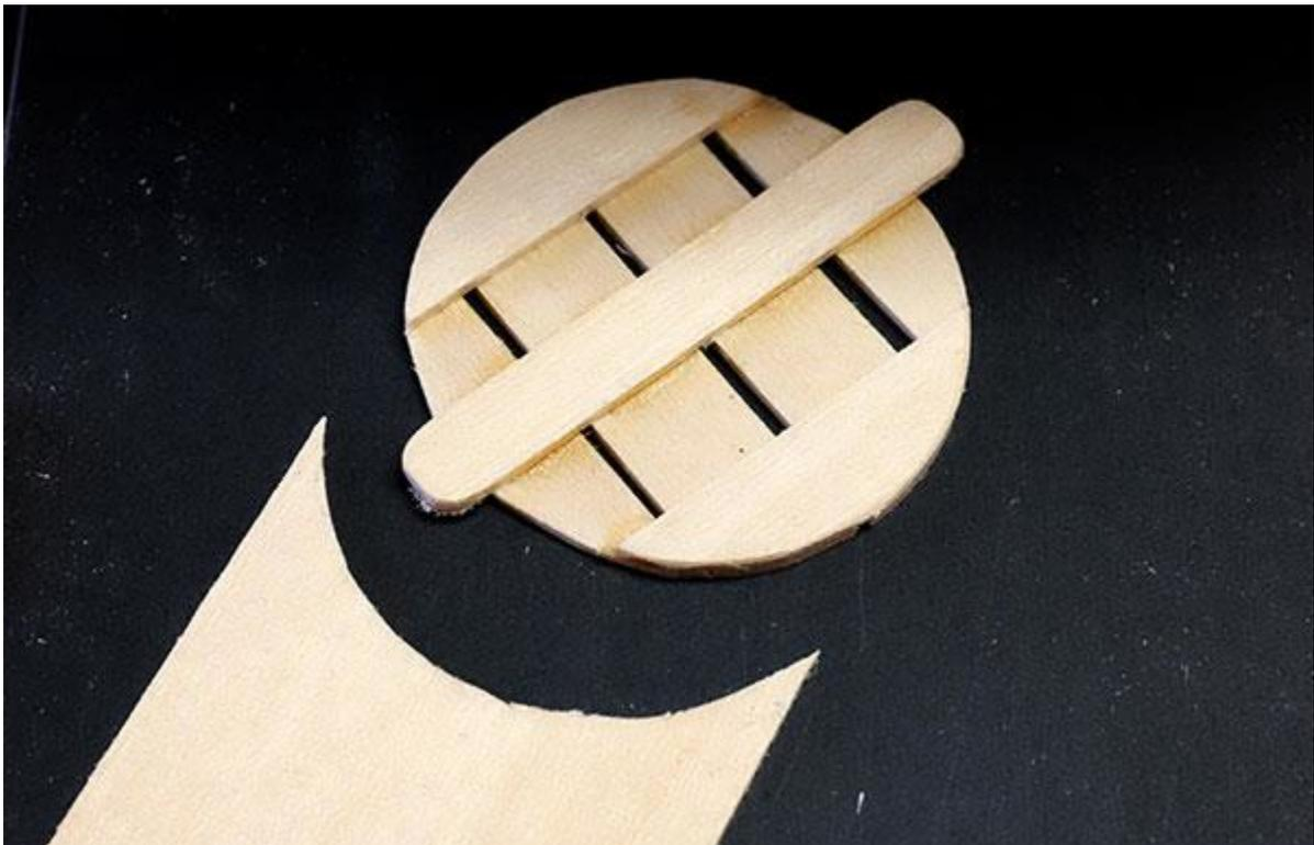
Now, you need a little shaping jig. It's nothing more than a piece wood with a narrower piece in the center. Clamp the lids down over the piece in the center so they get a nice curve to them. I wet the three cross pieces, then hit them with a hair dryer for a couple minutes. When they cool down, they'll hold that curve.
