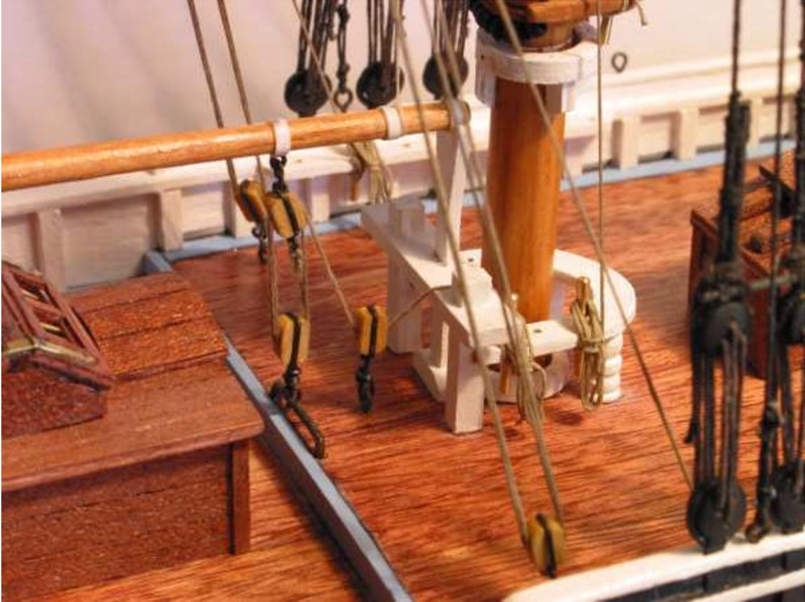
Photo 7: Fore sheet rigging and main fife rail and bitts.
