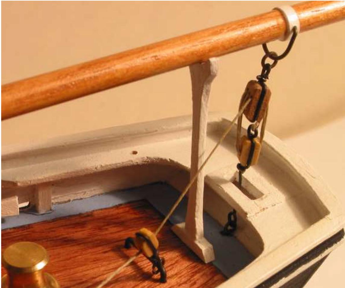
Photo 4: Main sheet and boom rest
