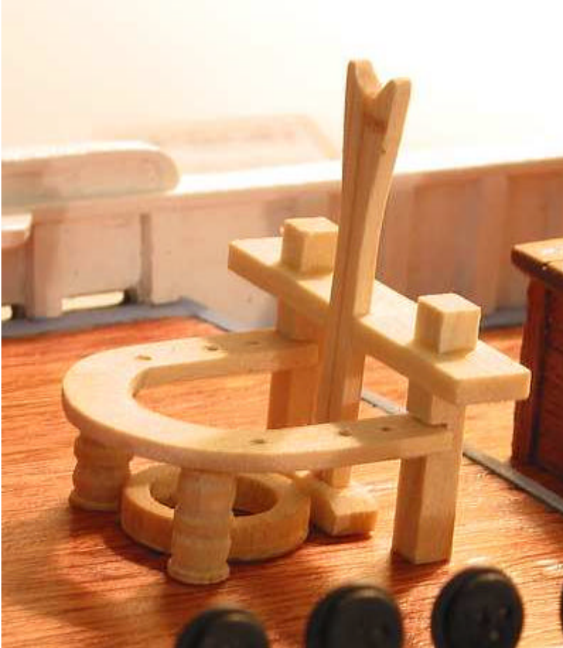
Photo 6: Main bitt and fife rail before painting
