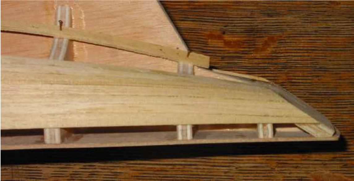
Photo 3: Placing the second planking batten
