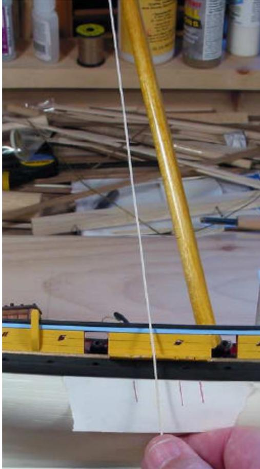
Photo 1: Aligning the chain plates
