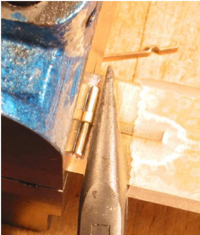
Photo 2: Shaping the cap irons.
