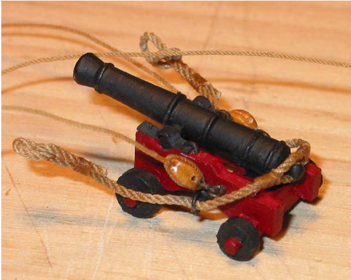
Photo 4: Cannon ready to install with breeching rope in place.
