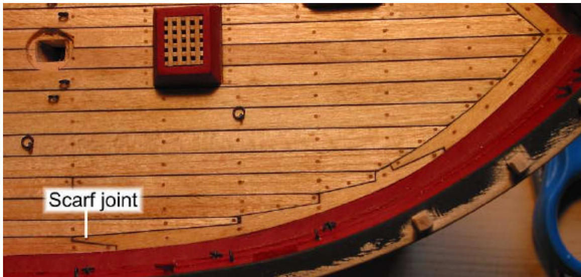
Photo 6: Scarf joints and nibbing
