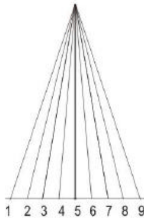
Diagram 1: Triangle for equally dividing segments
