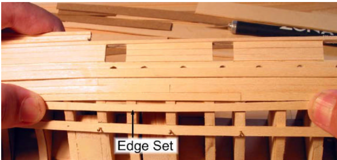
Photo 4: Edge setting a plank in the center of the boat.
