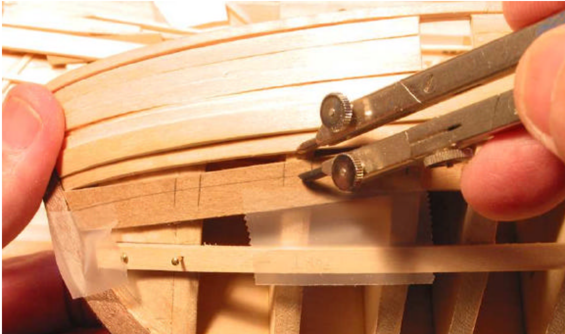
Photo 2: Marking the poster-board spiling template.
